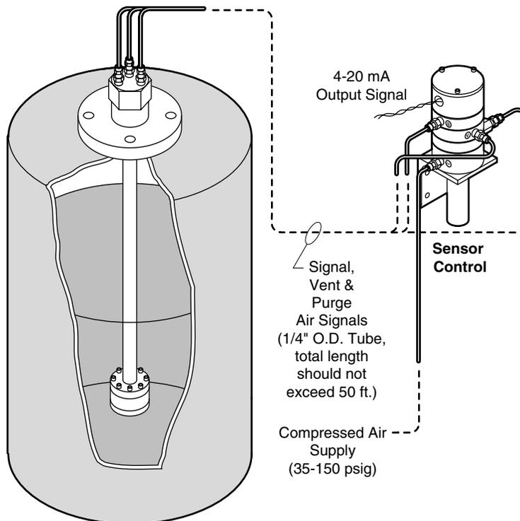
**Complete Sensor Package - Electronic 4-20 mA Output**
